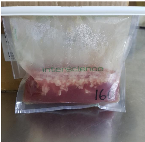
Figure 7B: Sealed plastic bag containing a 25 g homogenized sample in 225 ml buffered peptone water.
