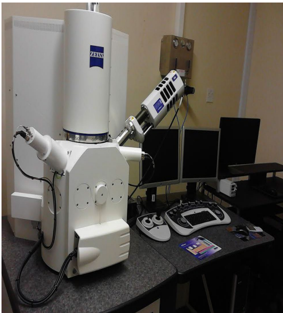
Figure 3. 2. (a) SEM of the University of Zululand in the Physics and Engineering Department. (b) Schematic illustration of the basic components of the SEM [9].
