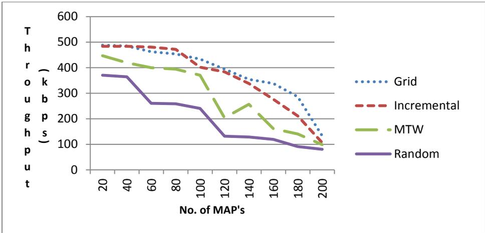
Figure 5.19 :Network Throughput when One MPP is deployed
