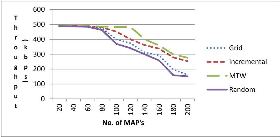
Figure 5.10: Network Throughput when One MPP is deployed
