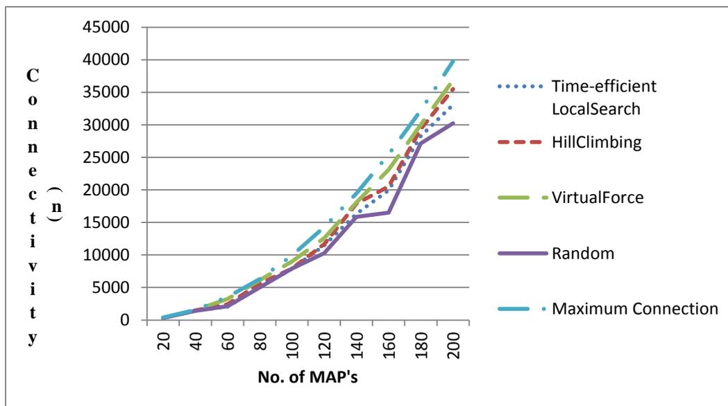
**Figure 4.15: Network Connectivity in Linear Settlement Pattern**
