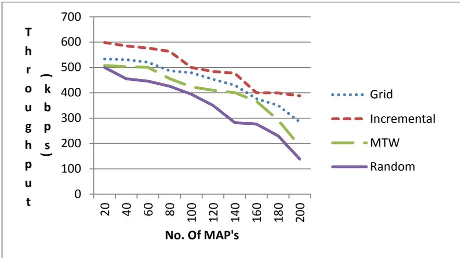
Figure 5.29: Network Throughput when Two MPP's are deployed
