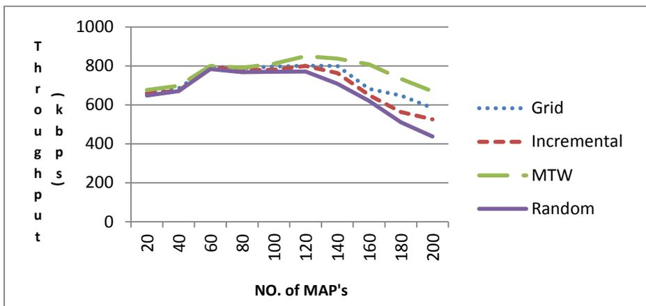
Figure 5.3 :Network Throughput when Three MPP's are deployed
