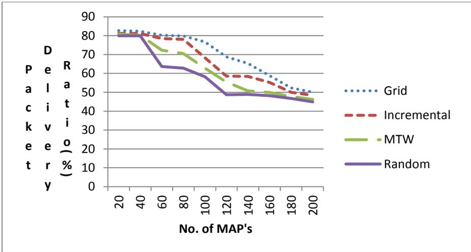
Figure 5.25 :Network packet delivery ratio when one MPP is deployed
