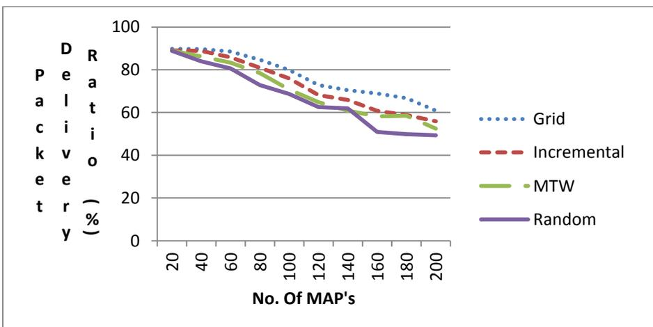
Figure 5.27 :Network packet delivery ratio when Three MPP's are deployed
