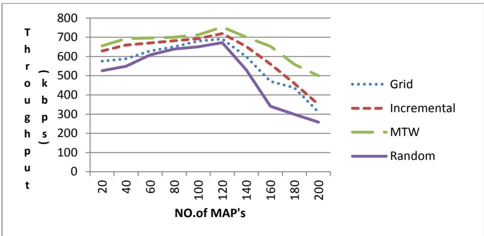
Figure 5.12: Network Throughput when Three MPP's are deployed
