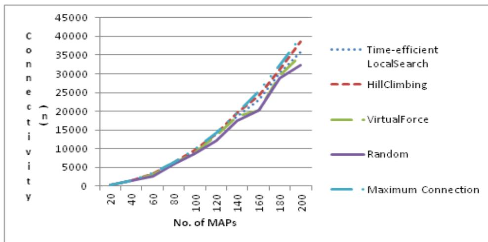
**Figure 4.3 Network Connectivity in Nucleated Settlement Pattern**
