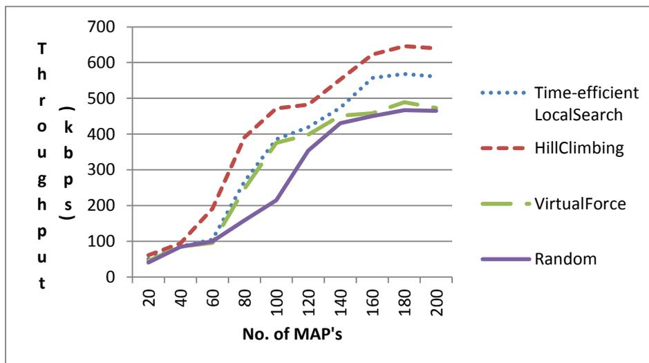
**Figure 4.4: Network Throughput in Nucleated Settlement Pattern**
