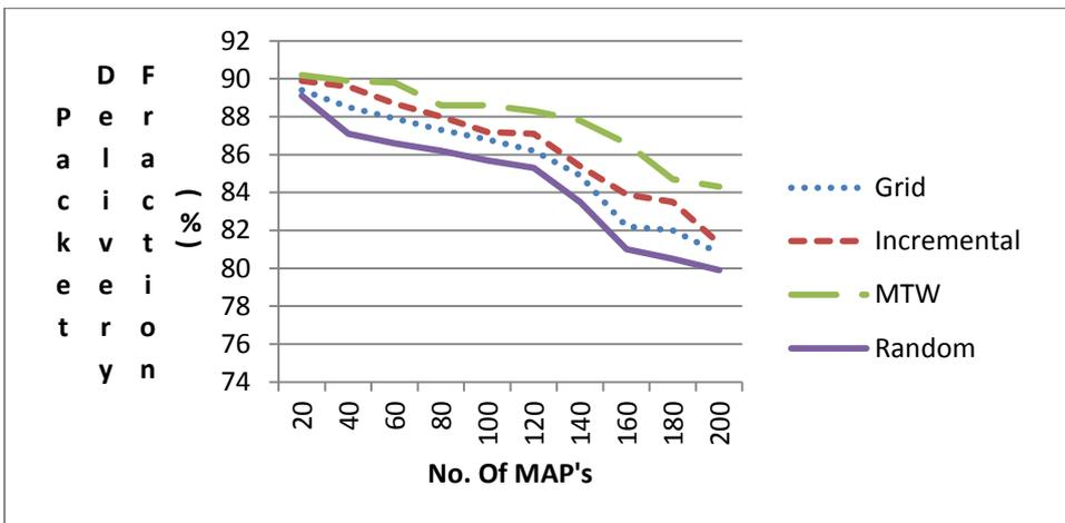
Figure 5.17: Network Packet Delivery Ratio when Two MPP's are deployed
