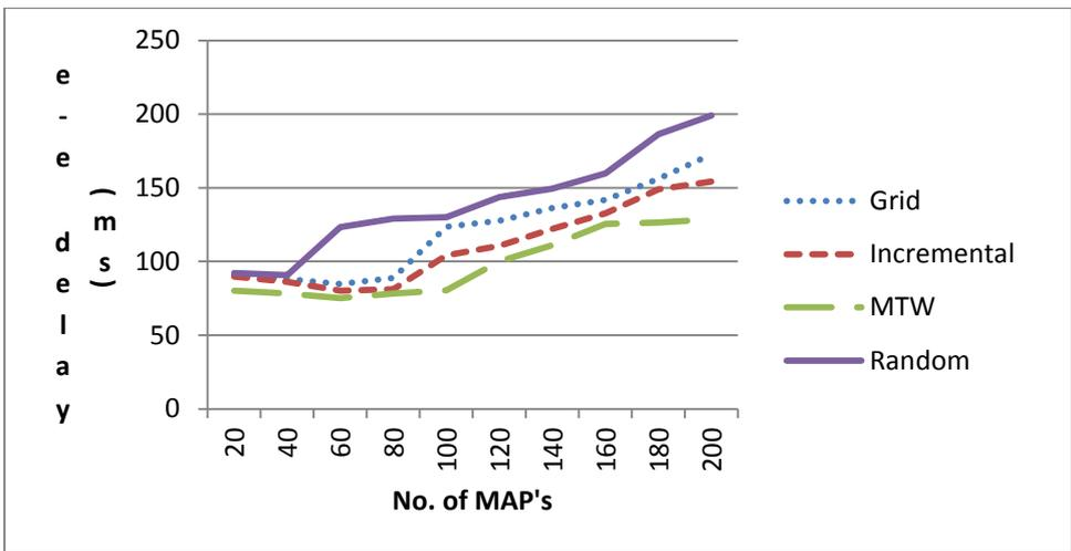
Figure 5.14: Network end-to-end delay when Two MPP's are deployed
