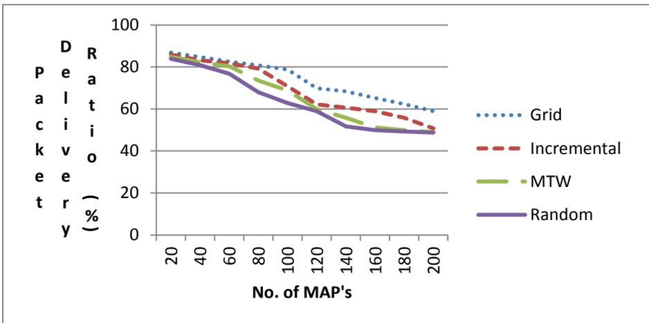
Figure 5.26: Network packet delivery ratio when Two MPP's are deployed
