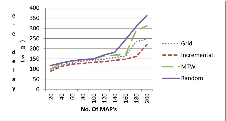
Figure 5.31: Network End-to-end Delay when One MPP is deployed
