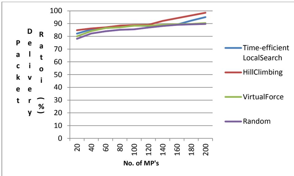
**Figure 4.6: Network Packet Delivery Ratio in Nucleated Settlement Pattern**
