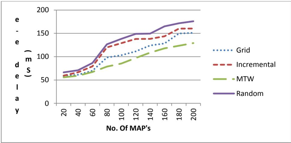
Figure 5.5: Network end-to-end delay when Two MPP's are deployed
