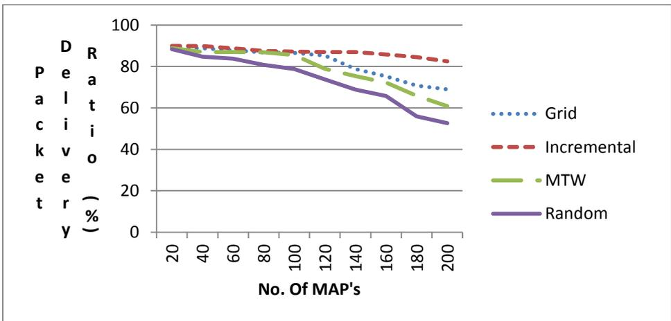
Figure 5.36: Network Packet Delivery Ratio when Three MPP's are deployed
