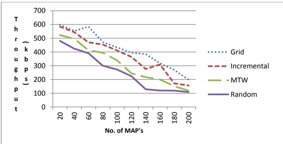
Figure 5.20: Network Throughput when Two MPP's are deployed
