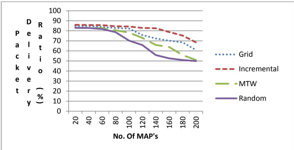
Figure 5.35: Network Packet Delivery Ratio when Two MPP's are deployed
