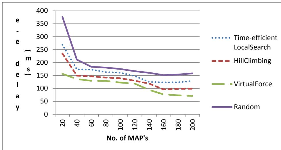
**Figure 4.17: Network end-to-end Delay in Linear Settlement Pattern**
