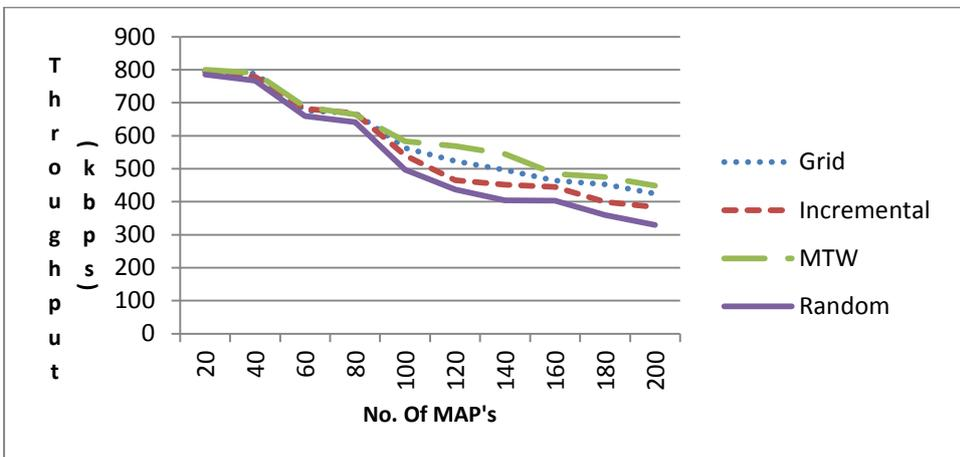
Figure 5.2: Network Throughput when Two MPP's are deployed
