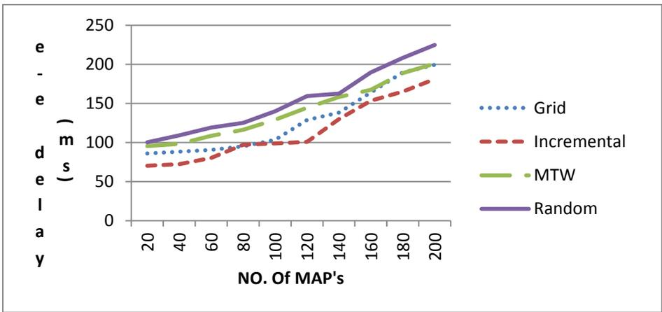
Figure 5.32: Network End-to-end Delay when Two MPP's are deployed
