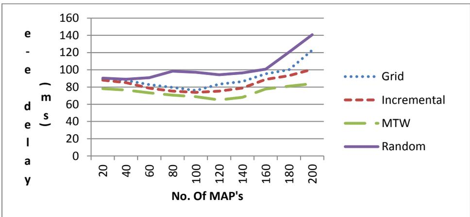
Figure 5.15 :Network end-to-end delay when Three MPP's are deployed
