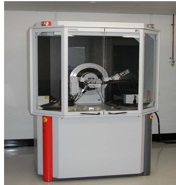
Figure 4.3 The schematic representation and the photo of x-ray diffractometer. The x-ray source produces x-ray radiation and interacts with the sample and detected on the detector.
