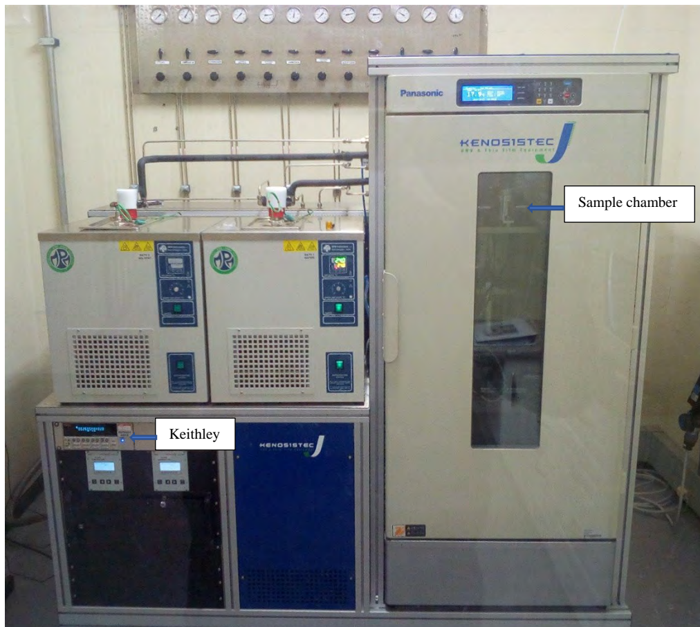
Figure 3. 11: KSGAS6S test system for gas sensors at UNIZULU.
