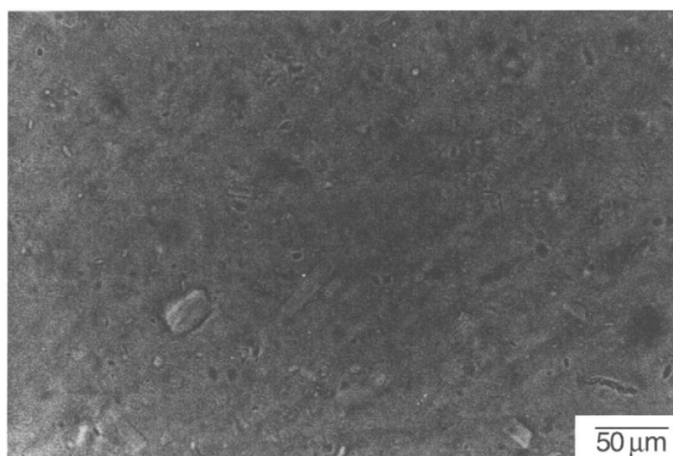
Figure 3.1: SEM image of green compact defects identified using the liquid immersion technique (Uematsu 1996)
