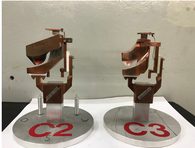
Figure 2.11: This picture shows the newly designed spiral inflectors that are used for 8 turns patterns in the SPC2 injector cyclotron.
