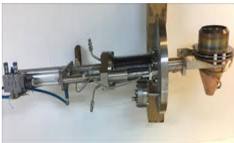
Figure 4.1: A picture of a Faraday cup used to measure beam intensity in the beam pipe [50].
