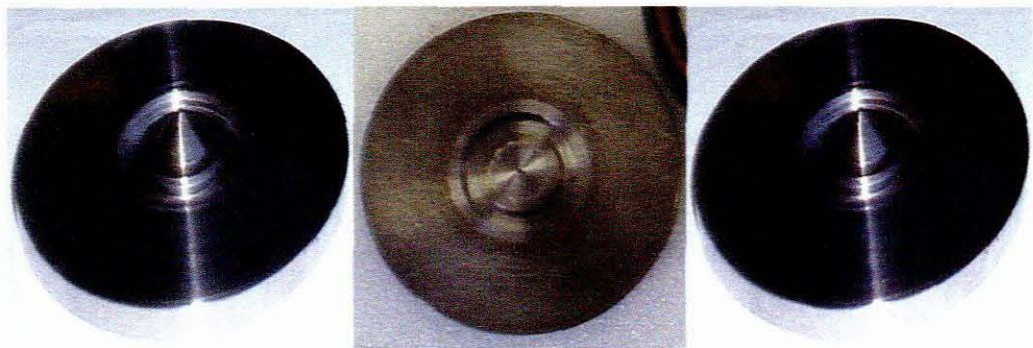
Figure 6.5: A pictures of the outlet electrode for different materials and shapes. The electrodes from left to right are: conical mild steel, flat mild steel and conical aluminium.
