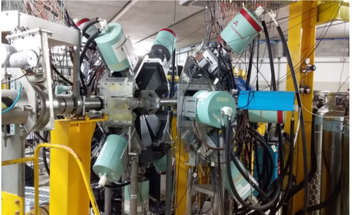
FIGURE 3.6: The iThemba LABS AFRODITE \gamma -ray spectrometer showing how the clover detectors were arranged in the experiment.
