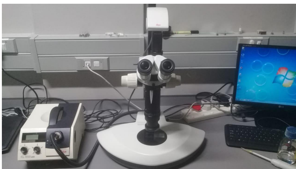
Fig. 4.4: The LEICA Z16 APO microscope. Crystals were viewed under this microscope which is attached to the SCHOTT KL 1500 LCD Fiber Optic Light Source.
