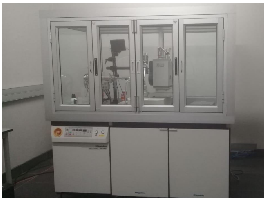
Fig. 4.5: X-ray generator (Rigaku MSC Micromax 007 dector). Crystals were diffracted for the detection of salt or protein crystals
