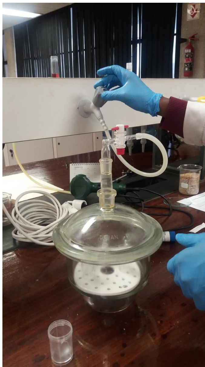
Figure 3.2: A glass vacuum dessicator. This was done to produce an ‘anaerobic’ protein solution to prevent any spurious heat interference caused by air coming out of the sample.
