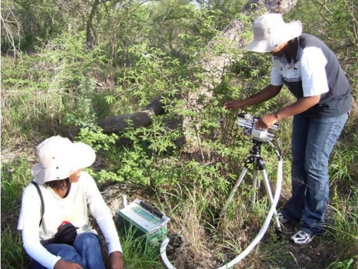
Figure 2.8: Li-Cor 6400 portable photosynthesis system was used to estimate photosynthesis on seedling of C. apiculatum in the full and non enclosure.
