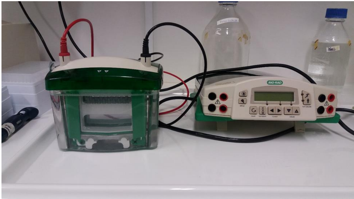
Figure 2.3: Mini-PROTEAN® Tetra Cell Systems and power pac™ used for gel electrophoresis.
