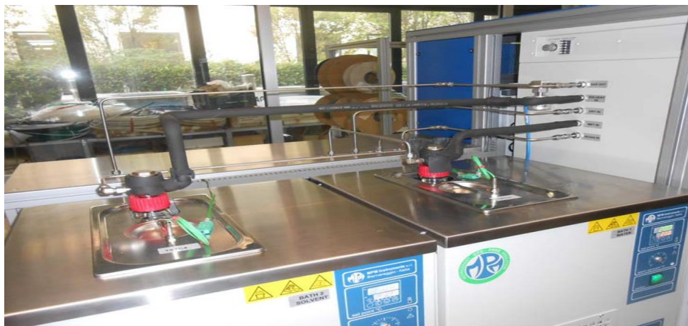
Figure 3.2.4.3: Thermostatic bath for generating humidity.
