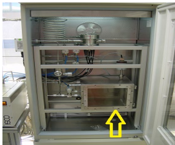
Figure 3.2.4.7: A special "de-gassing" chamber for solids (shown by means of a yellow arrow).
