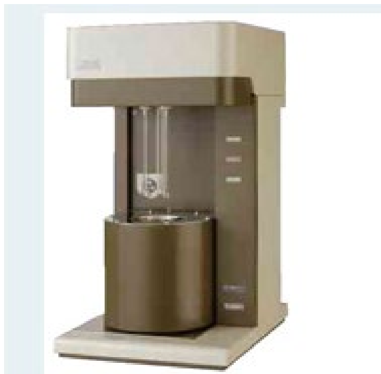
Figure 3.2.2.3: The BET instrument
