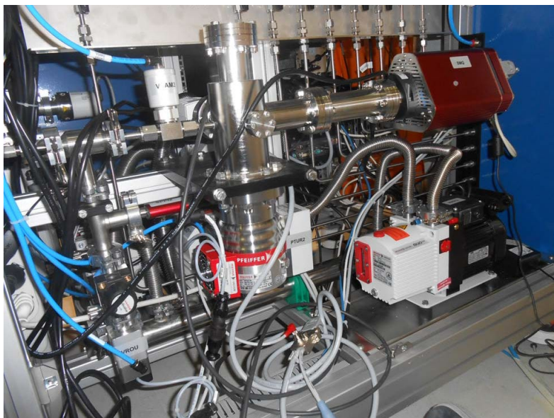
Figure 3.2.4.6: An RGA system with a mass spectrometer shown in red.
