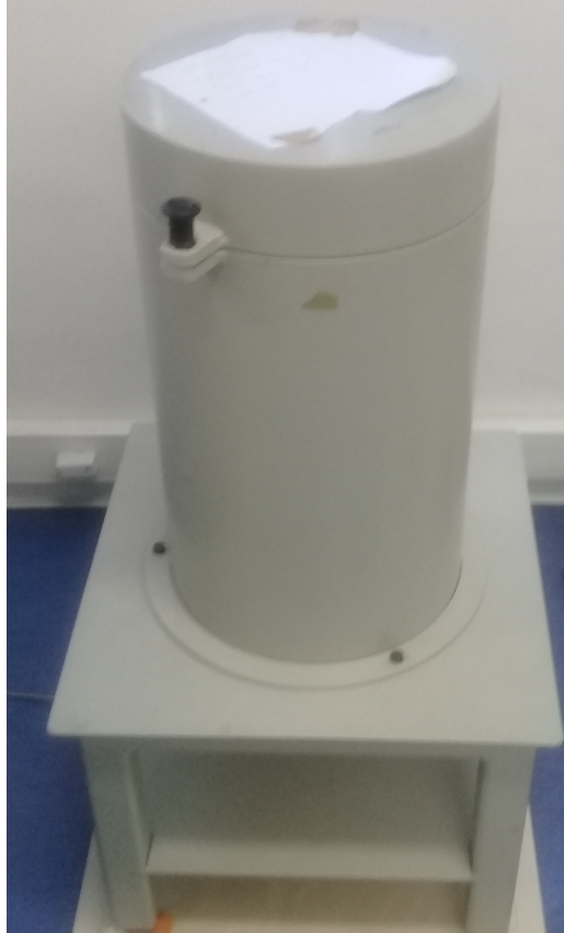
Figure 3.12: Lead castle that houses the NaI detector.
