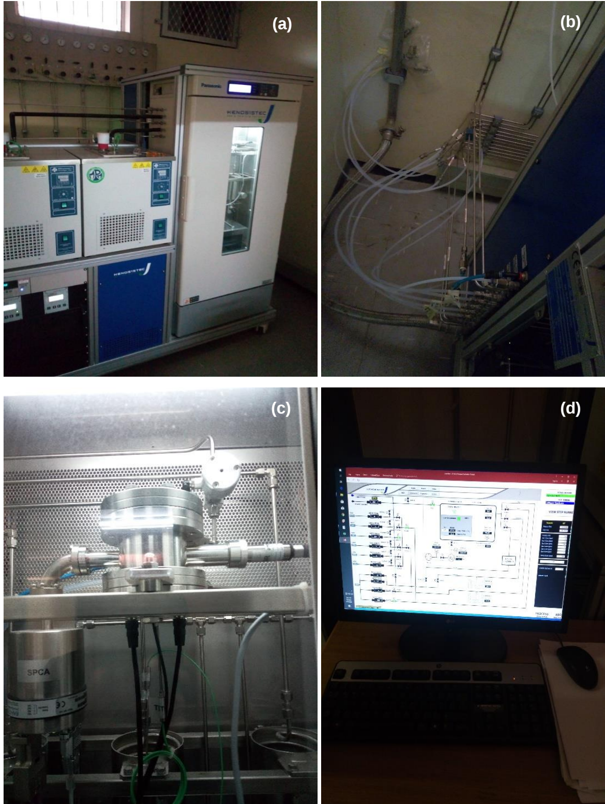
Figure 3.7. (a) KSGAS6S gas testing system, (b) gas lines, (c) the climatic gas testing chamber, (d) computer system.
