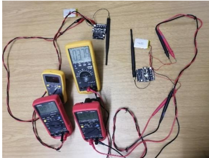
Figure 5.26 Low-Powered Devices with Multi-Meters Attached.
