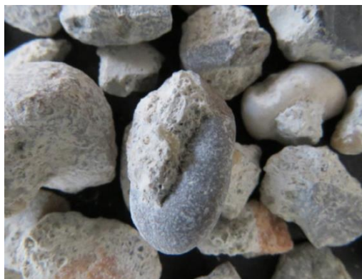
Figure 5.1. A pictorial example of recycled concrete aggregate sample with attached mortar paste [20].
