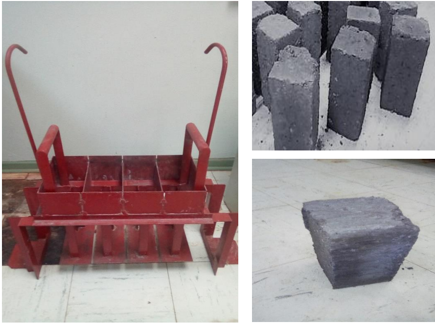
Figure 7.1: Laboratory mould presser and SCBA bricks developed
