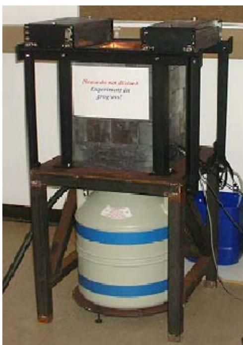
**Figure 3.8.** A photograph of the ERL iThemba LABS High Purity Germanium Detector.
