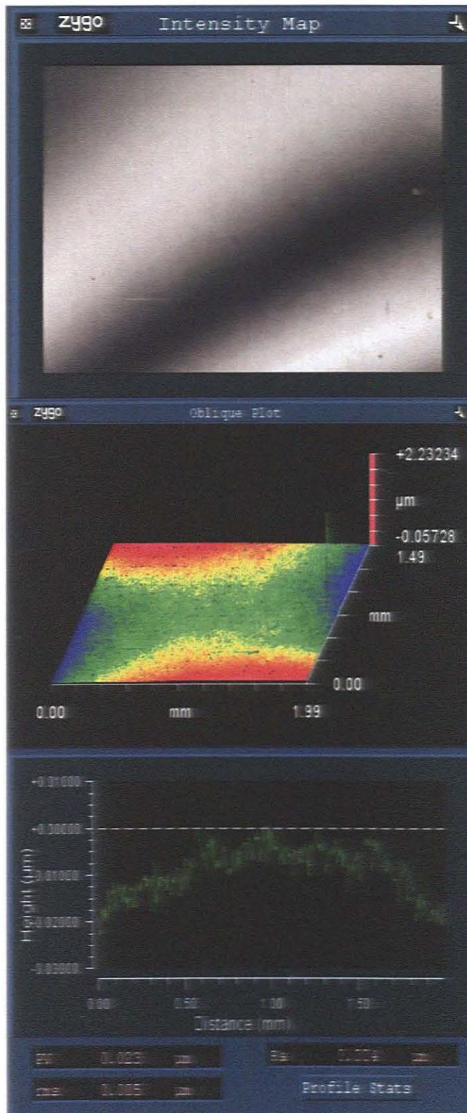
**Figure 25:** Typical interferogram obtained by Zygo interferometry (a) and in false color (b) as well as the deduced surface roughness profile (c).
