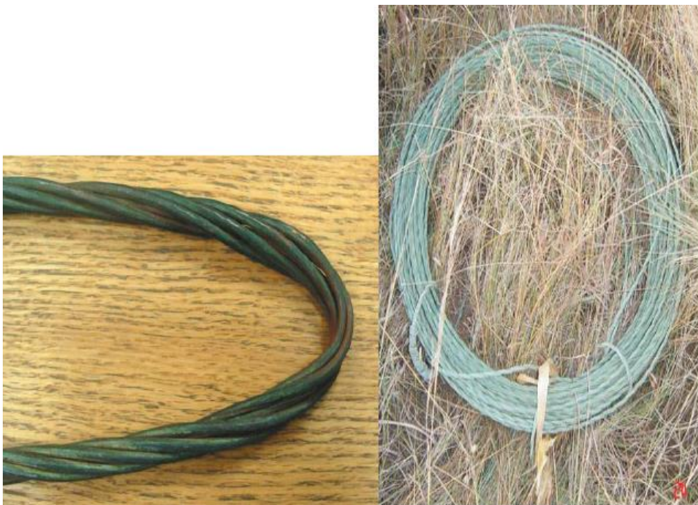
Figure A4.8: Copper conductors are used on overhead power lines.
