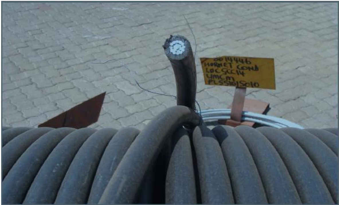
Figure A4.7: Covered aluminium conductor.
