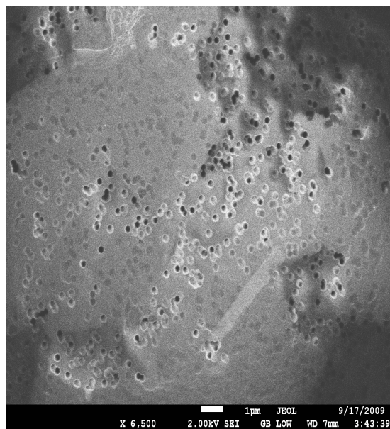
Figure 5-16 SEM micrograph of graphene sheet on track etch membrane revealing the ununiform distribution of the pores on the membrane.
