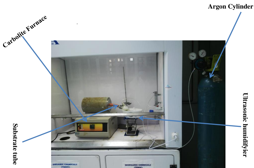
Figure 3.1: The AACVD setup during thin film deposition.
