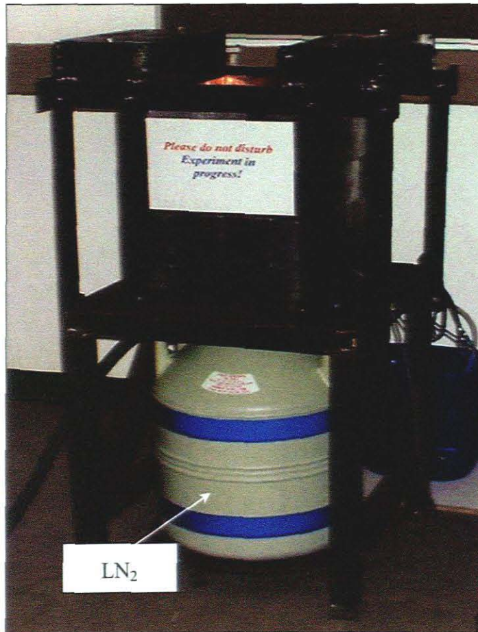
Figure 3-11: Photograph showing the lead castle of the ERL HPGe system, with the LN 2 dewar protruding underneath.
